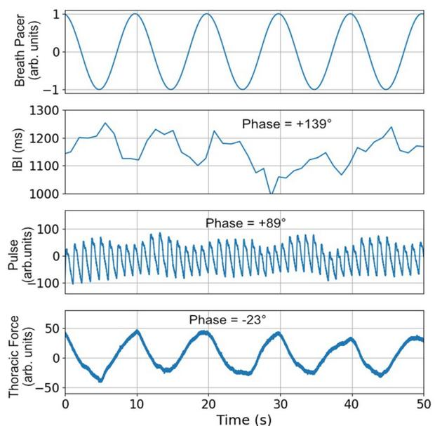
**Fig. 5** Dynamic Phase Extraction (DPE) can measure the phase and amplitude of the IBI Interval, Pulse Waveform, and Thoracic Force on a chest strap. In general, DPE can measure the phase and amplitude of any signal that is the same frequency as a reference signal. In this case, all phases are calculated with reference to the breath pacer
