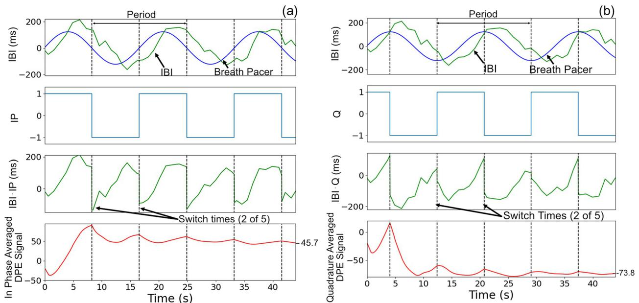
**Fig. 2** The Dynamic Phase Extraction (DPE) method extracts an In-phase Averaged Signal and a Quadrature (90 degrees out of phase) Averaged Signal. These are used to calculate the amplitude and phase
